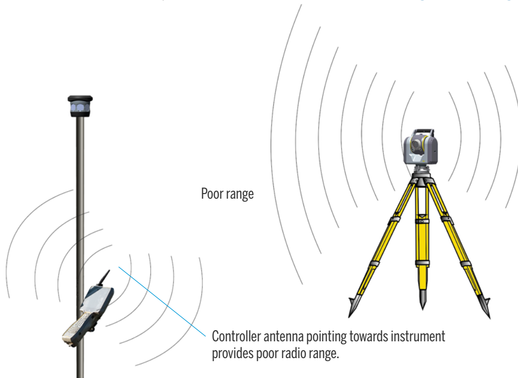
Figure 4.7 Poor radio range with controller antenna not in the same vertical position as the instrument antenna
