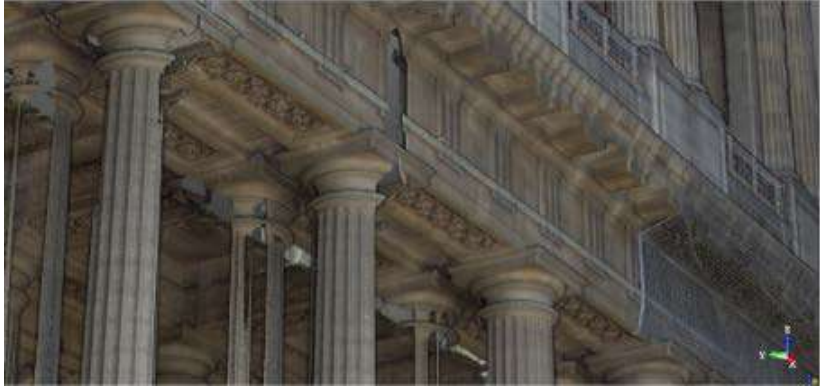
Point cloud displayed with the "Enhanced Ambient Shading" and "Adaptive Point Size"
